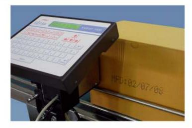
Simply attach the printer to your production line and start printing onto Carton, Tray, or other products, with excellent print quality.
